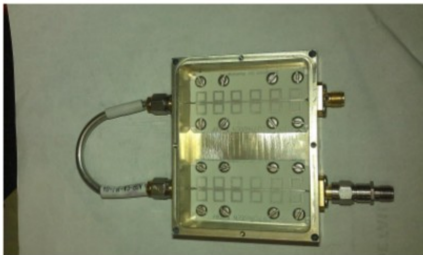
(c) Manufactured notch filter (with 6 dB attenuator to improve input match)
